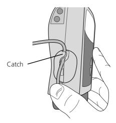
3. To seat the tubing into the groove, gently pull the tubing, until it is under the retention nubs and flat in the groove.
