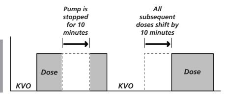
If you wish to make up for the lost time in the cycle, *it is recommended that you wait until the current dose is completed*. If the pump is stopped while a dose is infusing and you reprogram the "Dose Starts in" screen, then the pump will not deliver the remainder of that dose. (To determine the amount of time remaining in the current dose, use the Dose Remaining screen in the programming loop.) Then stop the pump, change to LL0 or LL1, and reprogram the delay on the "Dose Starts in" screen.
