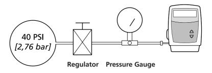
4. Connect the Medication Cassette<sup>™</sup> Reservoir outlet tube to the metered pressure source.
