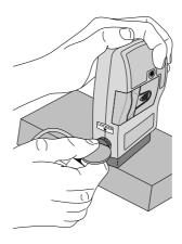
4. Insert a coin into the lock, push in, and turn counterclockwise until the line on the lock lines up with the arrow on the side of the pump and you feel the lock click into place.
