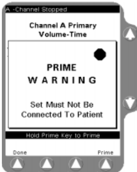
Figure 5-30 Ready to Prime
