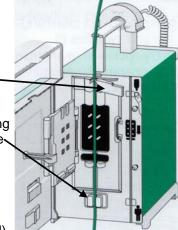
When the pump is turned on, it may display: **Tubing Type VISTA Pump Set** Confirm you are using a Vista™ Pump Set, then press **YES**.
