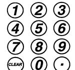
The numeric keys are used to enter values for any highlighted field requiring numeric data.
