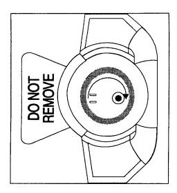
Turn the control knob on the cartridge to the closed position.
