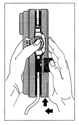
• Push cartridge into cartridge channel until firmly seated.
