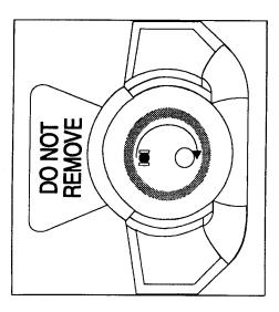
Confirm that the cartridge is in the open position with the dot inside the parallel lines.
