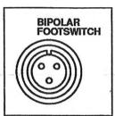
Connect a bipolar footswitch if you plan to use a footswitching bipolar instrument. You may use the footswitch to activate a handswitching instrument, if desired.
