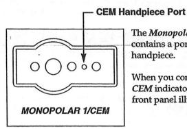
The *Monopolar 1/CEM* receptacle contains a port for connecting a CEM handpiece.
