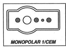
Insert the four-pin connector for the CEM handpiece into the *Monopolar 1/CEM* receptacle on the front panel.
