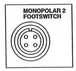
Connect a two-pedal monopolar footswitch to the *Monopolar 2 Footswitch* receptacle.
