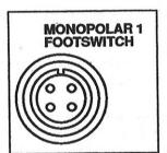
On the rear panel, insert the four-pin connector for the monopolar footswitch into the *Monopolar 1 Footswitch* receptacle.
