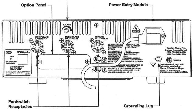
Some institutions require that electrosurgical generators be connected to protective earth ground, using an equipotential grounding cable. The Force FX is equipped with an equipotential grounding lug for that purpose.
