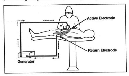
Monopolar electrosurgery is used for most surgical procedures. It is especially useful for procedures that require sparking to tissue, such as those in which tissue must be cut or coagulated over wide areas.
