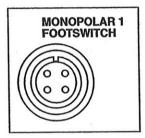
Connect a two-pedal monopolar footswitch to the *Monopolar 1 Footswitch* receptacle.
