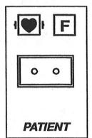
Insert the connector for the patient return electrode into the *Patient* receptacle on the front panel.
