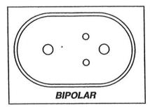
Connect a footswitching instrument with a two-pin connector.
