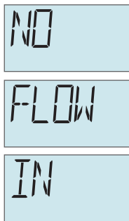
Figure 3-4 NO FLOW IN Alarm
