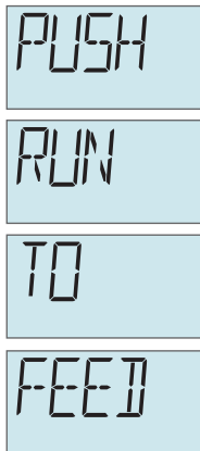
Figure 3-7 PUSH RUN TO FEED Alarm
