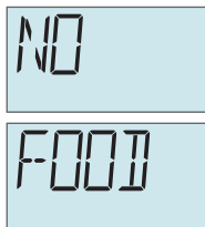
Figure 3-6 NO FOOD Alarm
