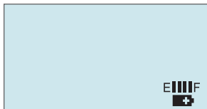
Figure 3-12 Battery Symbol and the E and F of the Fuel Gauge
