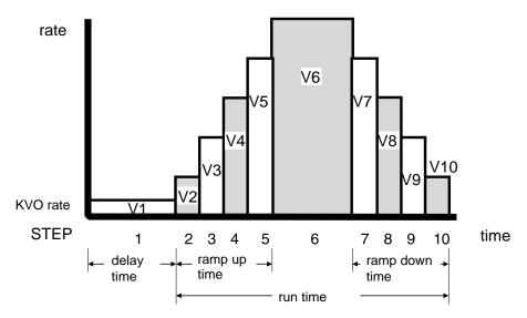
Figure 5. Sample Ramp Program Delivery Profile (PDP)
